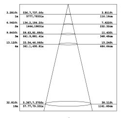
Note: The Curves indicate the illuminated area and the average illumination when the luminative is at different heights. Illumination values measured in footcondles, 1 Average output at a specified height relative to total output within  $\pm 10\%$  depending on device configuration
